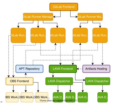
From the point of view of developers and product teams, GitLab is the main interface to Apertis. All the source code is hosted there and all the workflows that tie everything together run as GitLab CI/CD pipelines, which means that its runners interact with every other service.
