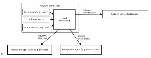
Thanks to the Wayland input flow only having two actors (the compositor and the receiver) (as opposed to that of X11) that there is no way for applications to either spy on the inputs of other applications or to inject inputs into other applications.
